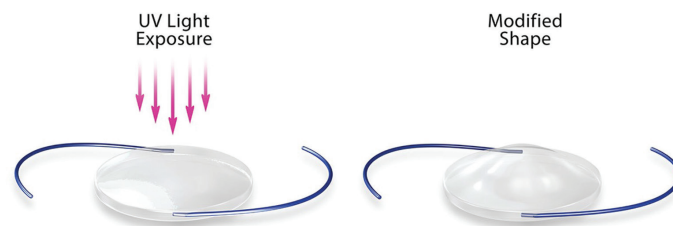
Figure 2. UV light exposure fine-tunes the final IOL power.
